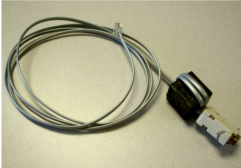
FIG 4. Ferrite Installation - to Host Computer
